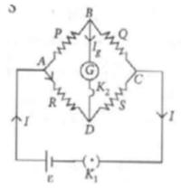
This is called the balancing condition. If any three resistances are known, the fourth can be found. The practical form of Wheatstone bridge is slide wire bridge or meter bridge. Using this the unknown resistance can be determined as  $S = \left(\frac{100-l}{l}\right) \times R$ , where l is the balancing length of the Meter bridge.
